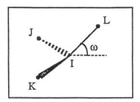
If omega0 = 0 the potential term has a minimum for the planar structure. Otherwise it has two minima at +/-omega0, with a barrier in between.
