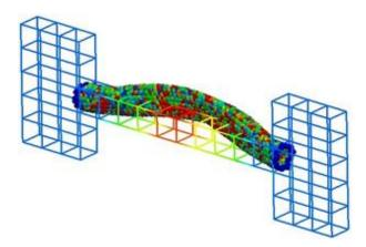
Interscale operators are defined that construct continuum fields from atomic data. Coupled simulations use FE projection approximated on a discrete field. Currently, coupling is restricted to thermal physics. The Hardy module can use either FE projection or integration Kernels evaluated at mesh points.
