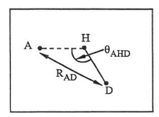
These 3-body interactions can be defined for pairs of acceptor and donor atoms, based on atom types. For each donor/acceptor atom pair, the 3rd atom in the interaction is a hydrogen permanently bonded to the donor atom, e.g. in a bond list read in from a data file via the read\_data command. The atom types of possible hydrogen atoms for each donor/acceptor type pair are specified by the pair\_coeff command (see below).
