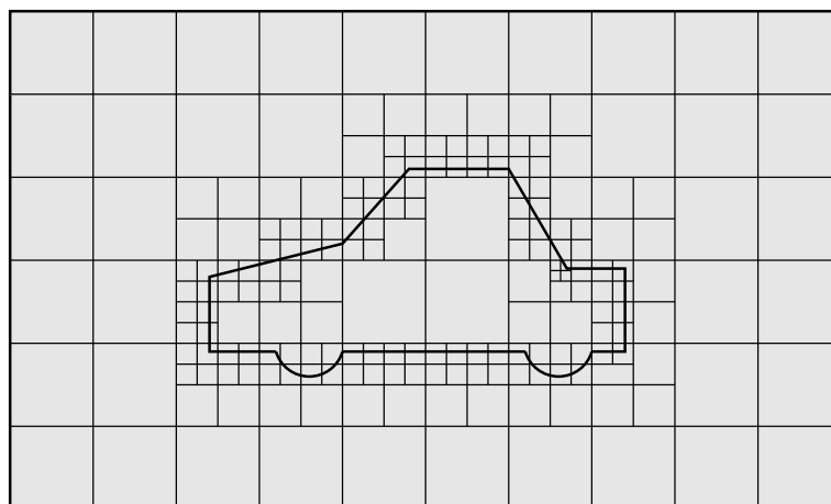
Figure 5.11: Cell splitting by surface in snappyHexMesh meshing process
